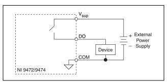
Figure 3. Connecting a Device to the NI 9472/9474
